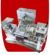
Inside the range, O.M.A.R. offers thermoforming machines that have a fundamental characteristic: blister quality in depth higher than the standard, which thermoform pockets from **27 mm** with BF 50 HT Model to **40 mm** with BF150 Model. This model of packaging machine is able to pack products such as flacks, ampoules and vials, meeting the request of the medical and dental industry. For this type of product the feeding area is
