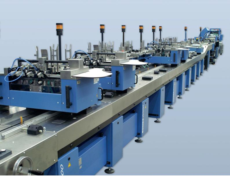
In developing the **4000 series of Poly & Paper Wrapping Systems**, Buhrs has produced a perfect combination of a low and ergonomic gathering section with mobile feeders, and a servo-driven wrapping module in combination with the Buhrs Data Controller (BDC).
