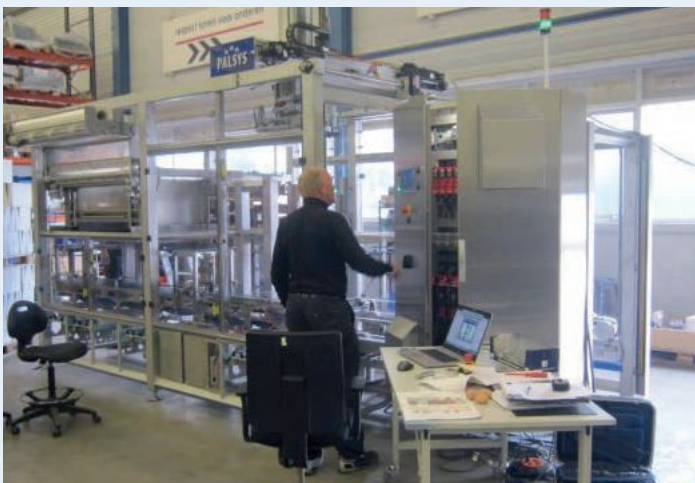
Under test: AISI304 palletiser with integrated automatic pallet magazine, sheet and foil dispenser and interlayer pallet placement.
