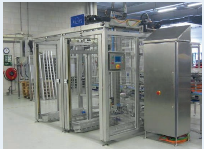
P40-AISI304 palletiser ready for acceptance test.
