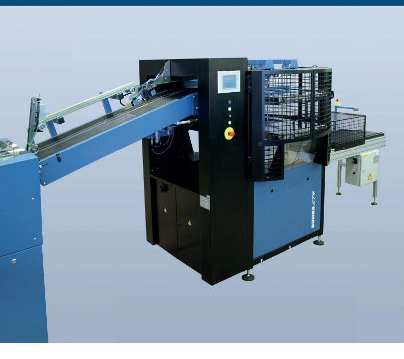
Buhrs has developed a new servo driven, highly productive compensating stacker. This new **Buhrs ST4 stacker** is specifically designed for handling wrapped and non-wrapped products.
