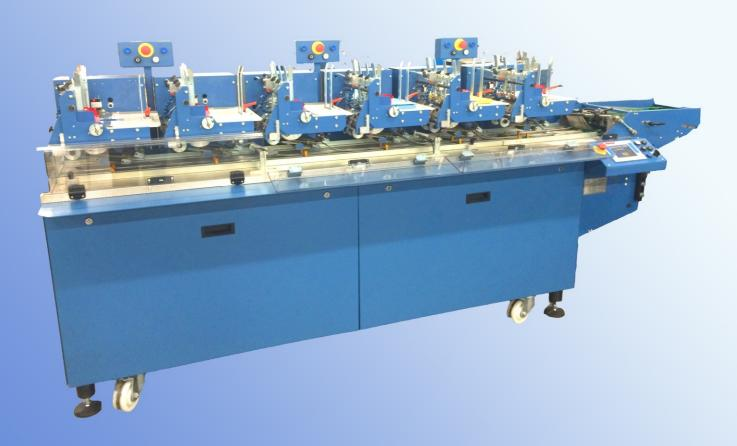
With **the mobile gathering section CS3000** you can optimize your system utilization. The CS3000 can easily be moved to the desired position with conveyor rollers and can be leveled with levelling feet in your production hall.
